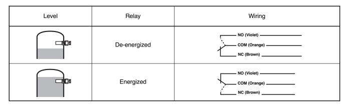
IMPORTANT: When power is lost or gap is dry; the relay de-energizes.
